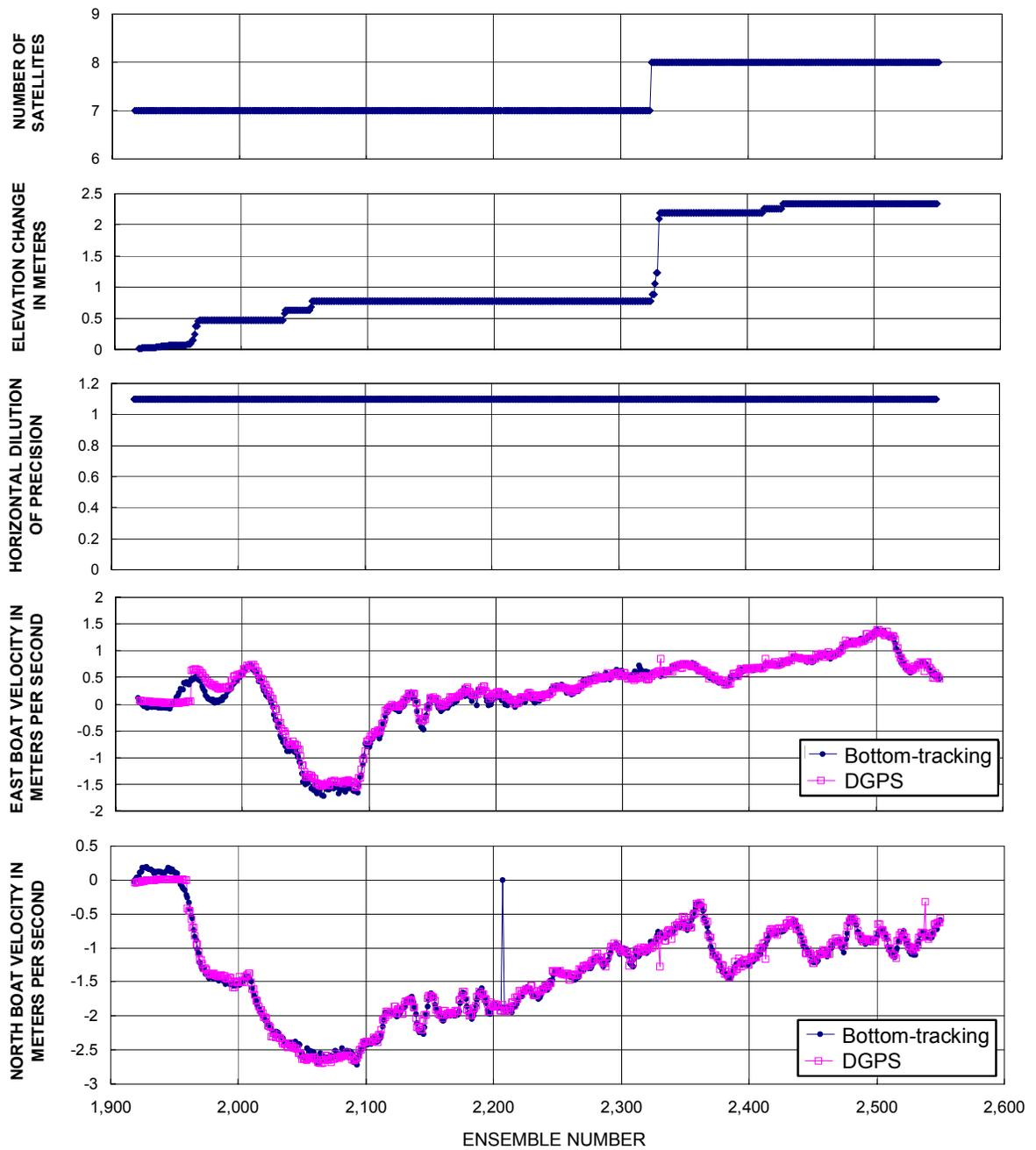
Figure 5. Comparison of differential global positioning system- and bottom-tracking-referenced boat velocities with differential global position system data-quality indicators for data collected on the Ohio River near Louisville, Kentucky.
