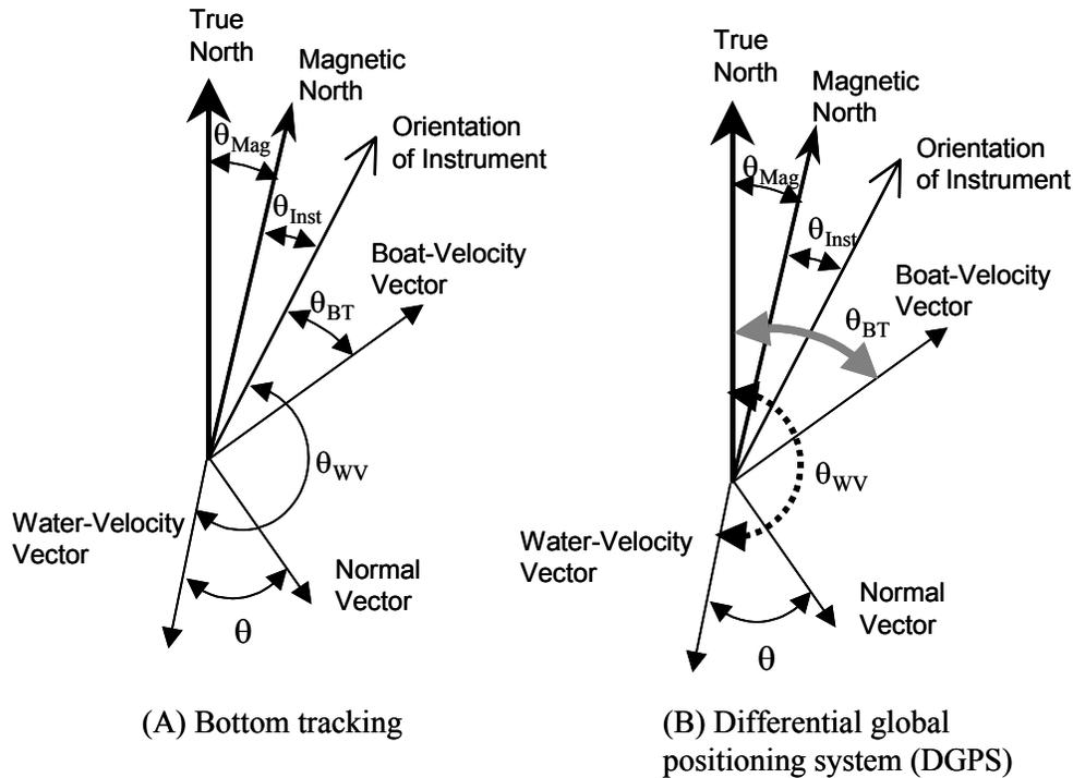
Figure 3. Vectors illustrating the difference between bottom-tracking and differential global positioning system (DGPS)-referenced boat-velocity vectors.
