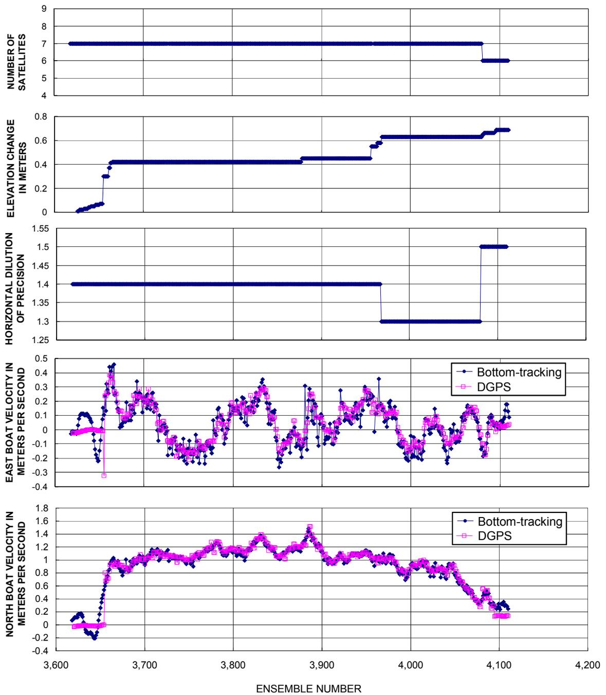
Figure 4. Comparison of differential global positioning system- and bottom-tracking-referenced boat velocities with differential global position system data-quality indicators for data collected on the Missouri River at Hermann, Missouri.
