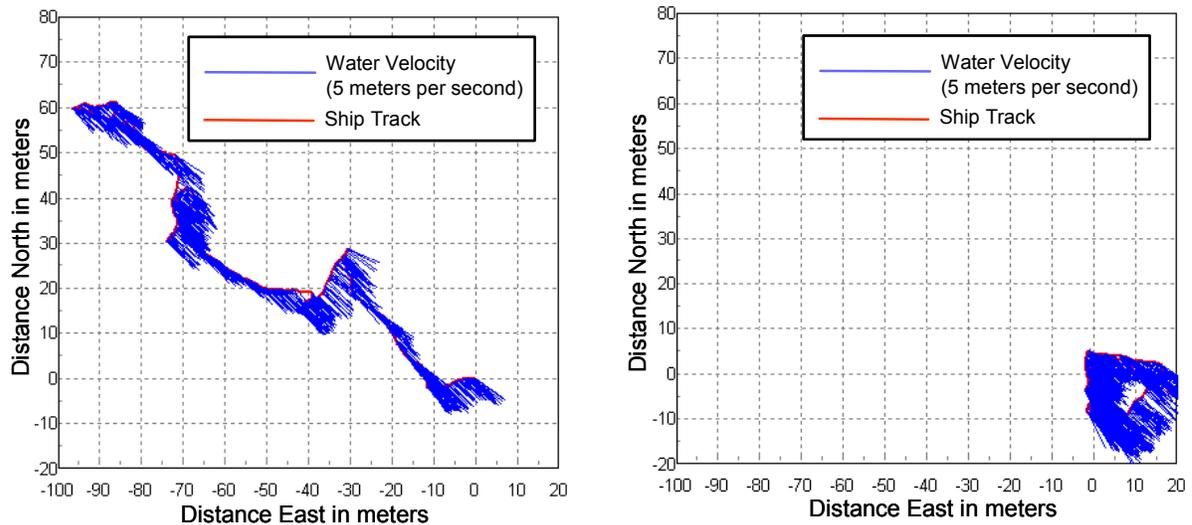
Figure 1. Example of a moving bottom measured with a 1,200-kilohertz acoustic Doppler current profiler on the Mississippi River at Chester, Illinois.
