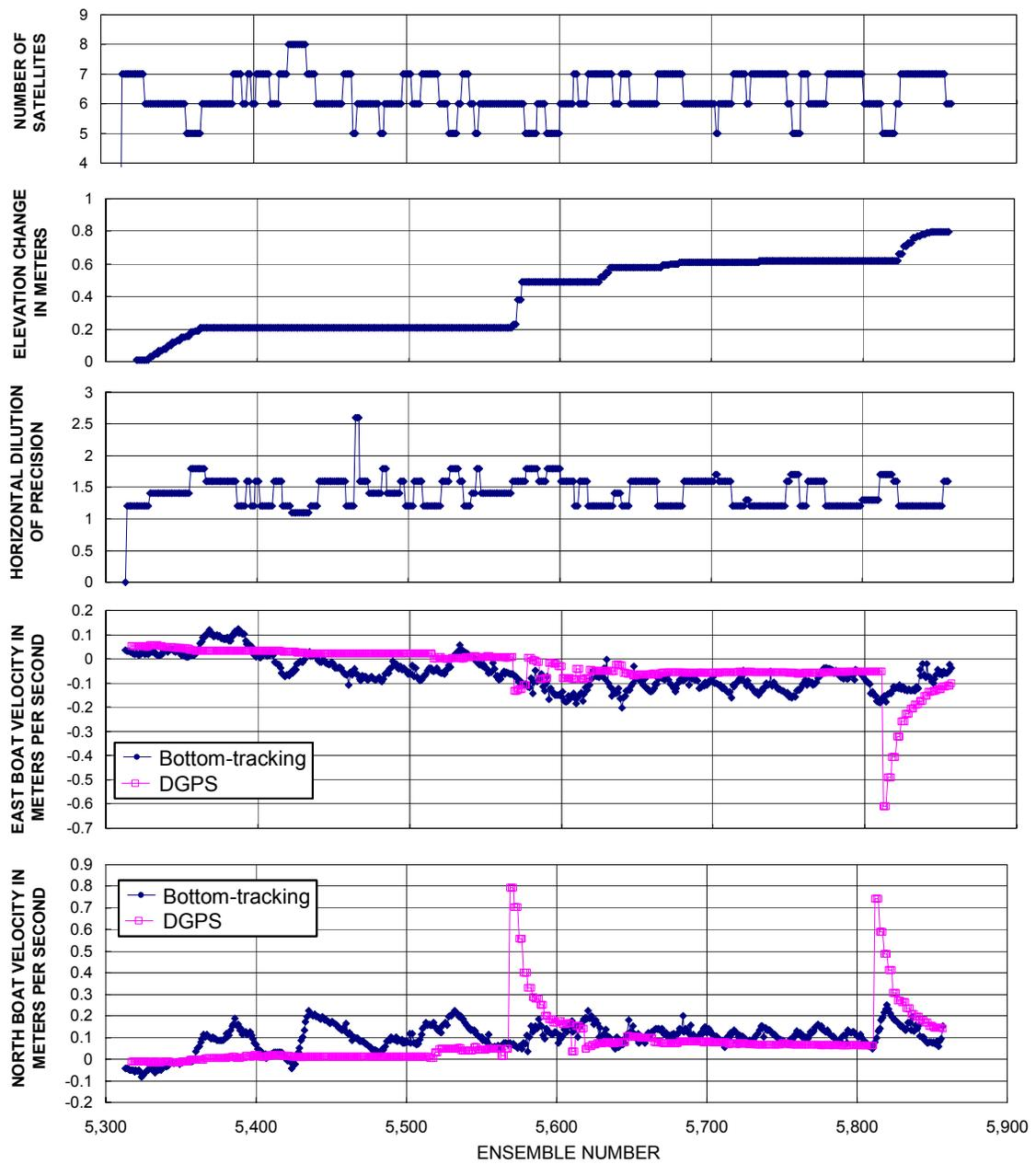
Figure 6. Comparison of differential global positioning system- and bottom-tracking-referenced boat velocities with differential global position system data-quality indicators for data collected on the Kankakee River at Dunns Bridge, Indiana.
