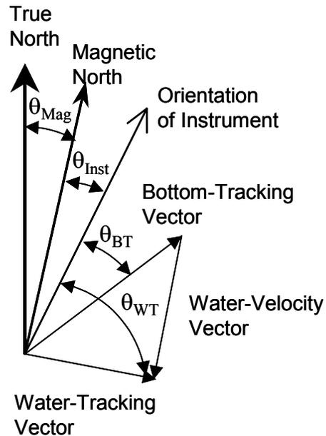
Figure 2. Vectors for computing the water-velocity vector.
