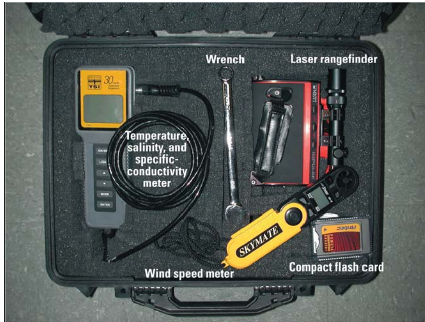
Figure 6. Example toolkit of ancillary equipment for use with acoustic Doppler current profilers (ADCPs) when making streamflow measurements. (Photograph by John M. Shelton, U.S. Geological Survey.)
