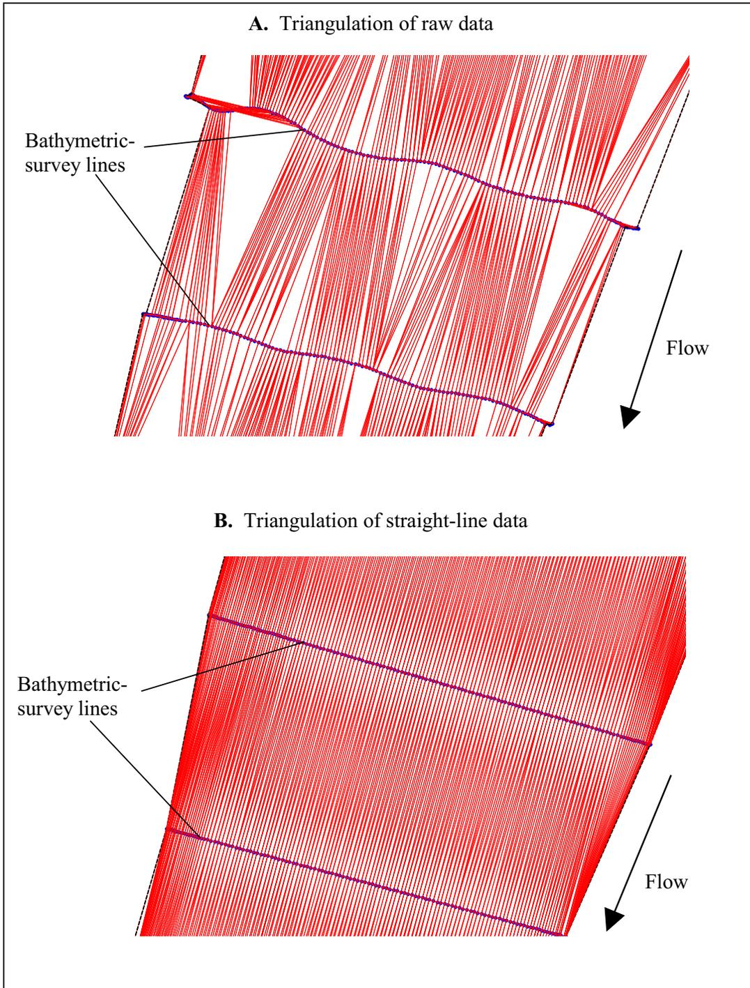
**Figure 5.** Surface Water Modeling System (SMS) software triangulation of raw and straight-line bathymetry data for a section of the upstream study reach in the Ohio River model simulation near Louisville, Kentucky.
