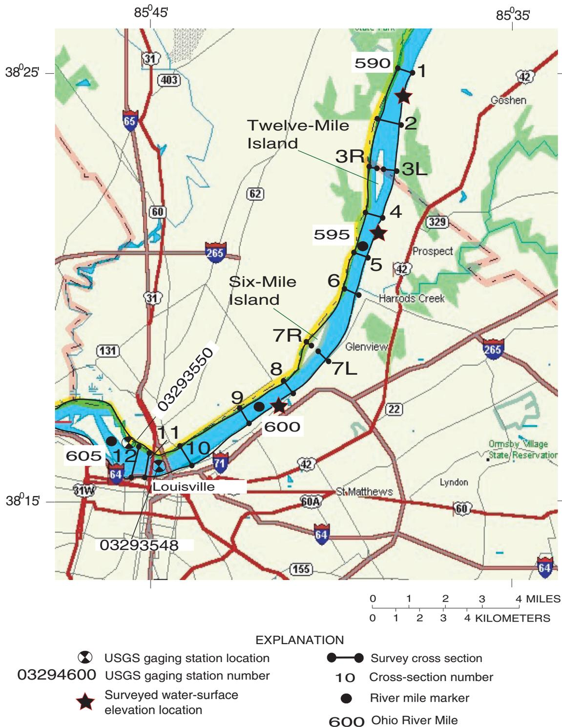
**Figure 3.** Location of hydrographic-survey cross sections, surveyed water-surface elevation stations, and U.S. Geological Survey (USGS) gaging stations in the upstream study reach near Louisville, Kentucky.
