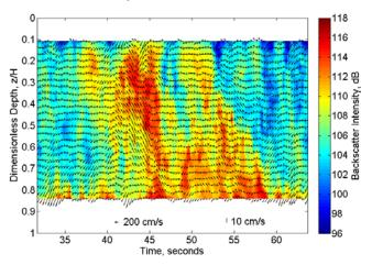
Figure 5. Backscatter intensity contours with streamwise and vertical velocity vectors in the upper lee of the dune.
