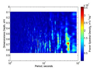
Figure 10. Power spectral density of streamwise velocity in the lower lee of the dune.
