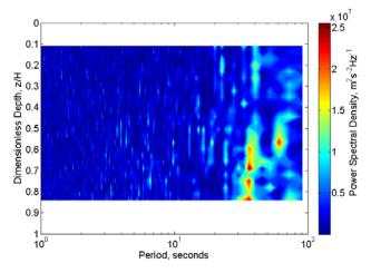
Figure 11. Power spectral density of streamwise velocity in the upper lee of the dune.
