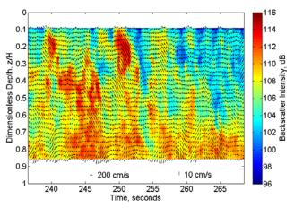
Figure 4. Backscatter intensity contours with streamwise and vertical velocity vectors in the lower lee of the dune.
