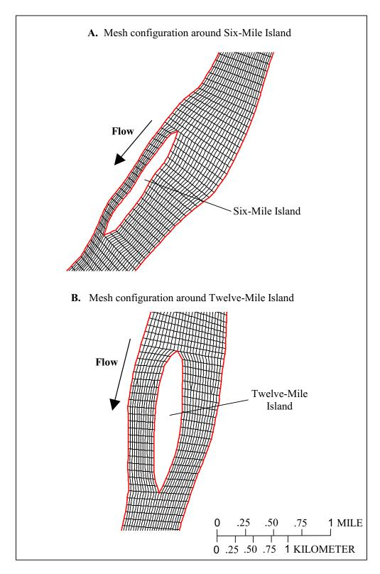
**Figure 7.** Mesh configurations around Six- and Twelve-Mile Islands in the upstream Ohio River study reach near Louisville, Kentucky.
