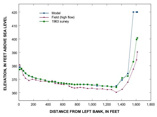
Figure 19. Comparison of cross-section 20 bathymetry in the downstream Ohio River study reach near Louisville, Kentucky.
