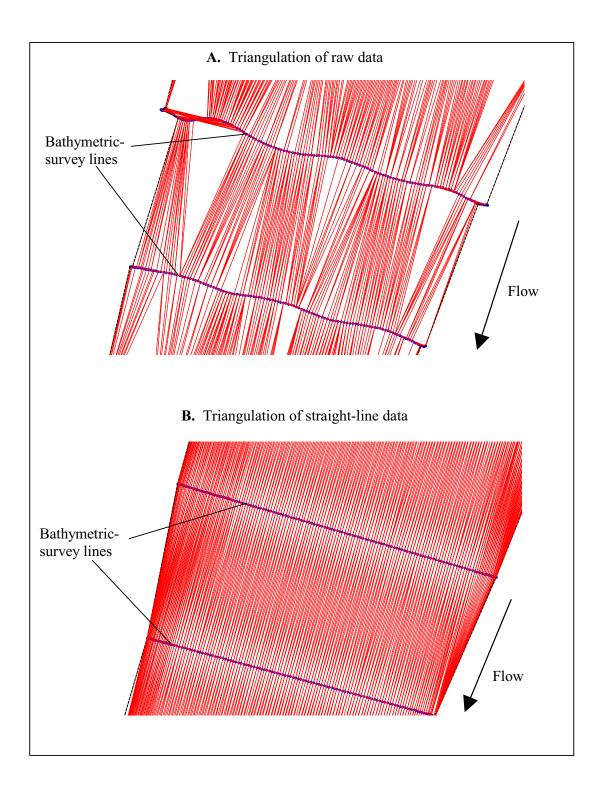
**Figure 5.** Surface Water Modeling System (SMS) software triangulation of raw and straight-line bathymetry data for a section of the upstream study reach in the Ohio River model simulation near Louisville, Kentucky.
