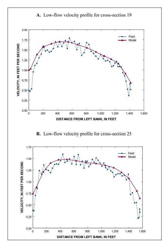
Figure 16. Field-measured and model-simulated low-flow velocity profiles for cross-sections 19 and 25 in the Ohio River model simulation near Louisville, Kentucky.
